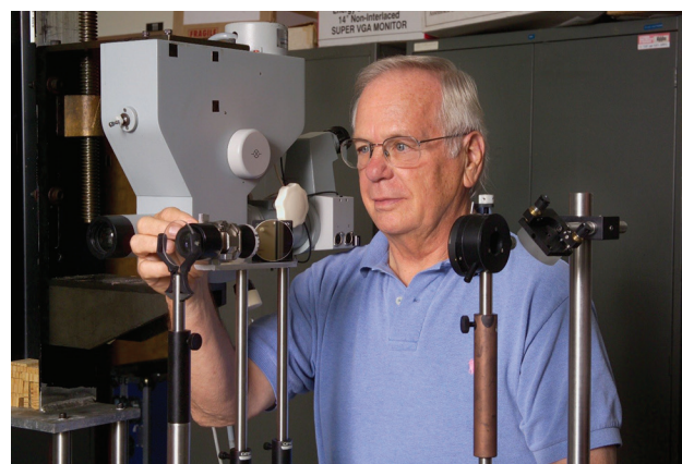
Figure 1-6. D. Jack Lund adjusts an optical element in one of the many optical delivery systems he developed to expose the eyes of animal models so that injury thresholds for a wide range of exposure conditions and response criteria could be measured. These data were the basis for setting safe exposure limits for humans. D. Jack Lund, in collaboration with his son, Dr Brian J. Lund (not pictured), were the first to measure retinal response thresholds with and without wave-front correction in support of the safety analysis of advanced, high-resolution retinal imaging systems.
