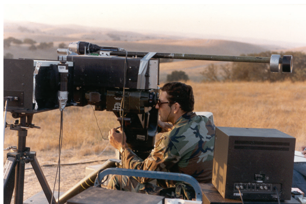
Figure 1-3. Major George Mastroianni observes laser glare from a moving Bradley fighting vehicle, at a range of 1,600 m, through the TOW (tube-launched, optically tracked, wire-guided) missile tracking device modified to measure tracking error. Although the laser glare was below the exposure limit, the exposure obscured the target during bright ambient daylight, which resulted in an off-target response.
